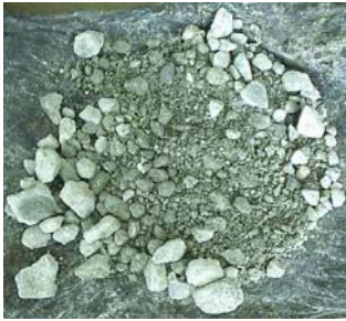
Serpentinised rubble and grit flushed from 7W
